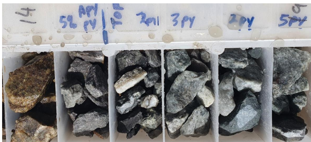
Figure 2: Hole BCRC011 chip tray interval at 14m to 20m drill depth, quartz and sulphide (variable 2% to 5% aggregate sulphide content with combined pyrite and arsenopyrite mineralisation) at base of oxidation - pending assay
